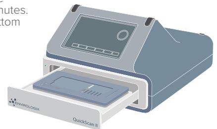
Read promptly by inserting the strip into the QuickScan and clicking "Read Test" on the Main Menu.
